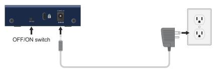
Note: Move the OFF/ON switch to the **ON** position to provide power to the device.
